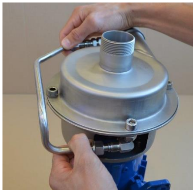
Fig. 3.5.6 Remove the metal pipe [1363].
