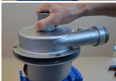
Fig. 3.5.12 Take off the pump casing [136].
