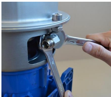
Fig. 3.5.7 Unscrew and remove the elbow union [1367].
