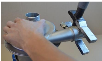
Fig. 3.5.8 Unscrew the connection adaptor [1364].
