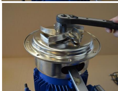
Fig. 3.5.14 Remove the impeller mounting screw [191] and the washer [192], use a spanner key in the opening of the pump back cover [1146] to hold the shaft [16Z] during assembly and disassembly of the impeller. Remove the impeller.
