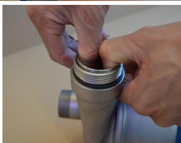
Fig. 3.5.9 Take out the strainer [1361] and the O-ring [1365].
