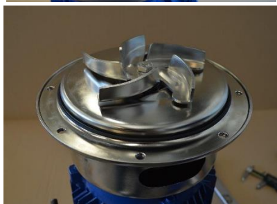
Fig. 3.5.13 Remove the O-ring [18]. NOTE! After every disassembly the O-ring [18] has to be replaced by a new one.
