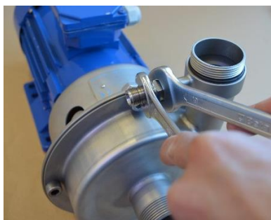
Fig. 3.5.10 Unscrew the straight union [1366].
