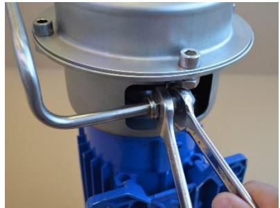
Fig. 3.5.5 Loosen the screw on the elbow union [1367].
